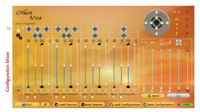
Configurations are presets that you can determine and which form the basis of a session being created: Use the various controls on the configurations mixer – you can set the light-emitting properties of the eight LEDs and then save them.
