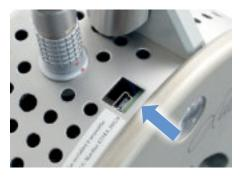
Lucia N°03 can also be connected via a USB cable (USB-plug adapter **22** at the lamp head) to the laptop. No further steps are necessary, because the laptop will automatically detect Lucia N°03.
