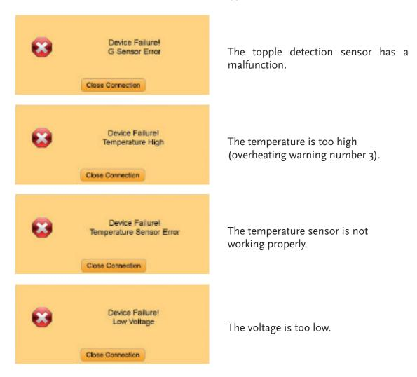
Click on **Close Connection** to disconnect. Unplug the power source, wait a moment (about 10 seconds) until Lucia N° 03 is completely powered off, then reconnect to the mains.
